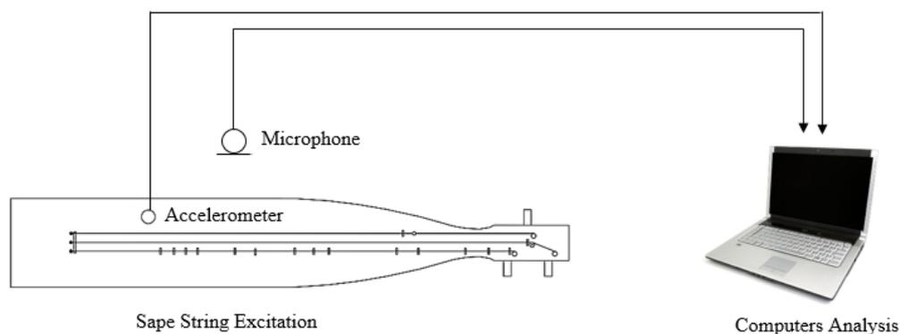
**Figure 3:** Experimental setup for the sound and vibration recording, and data analysis.
