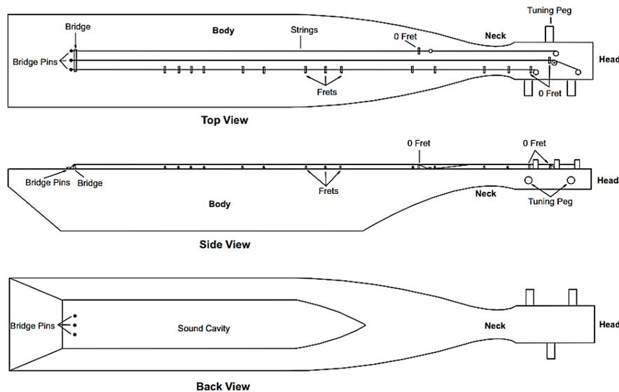
**Figure 1:** Schematic Drawing of sape
